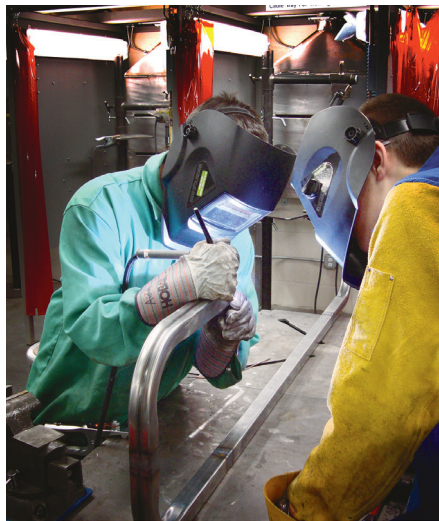
Walla Walla Public Schools SEA-Tech students TIG welding. Photo courtesy of Walla Walla Public Schools.
